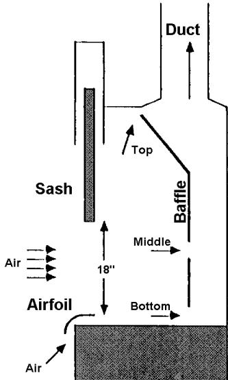
Figure showing common baffle locations
