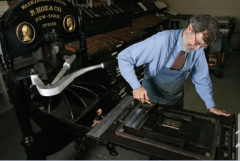
Mathews (left) inks a block in the studio, while students Derrick Austin '11 (left) and Victoria Alt '08 (right) set type by hand from a type case using composing sticks.
